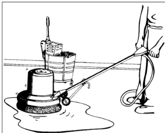
Figure 4. Applying the Statguard® Low Residue Floor Stripper with a scrubbing machine
